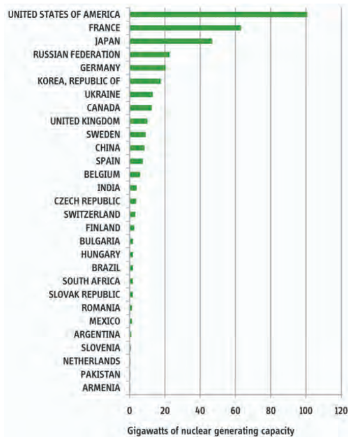
Figure 14.5 | Capacities of nuclear power reactors in operation by country, end of 2009. Source: data from IAEA-PRIS, January 9, 2010.
