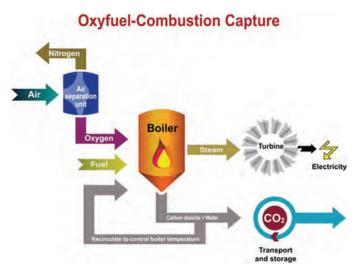
**Figure 13.3a-c** | Schematic showing the major steps and materials flows associated with the (a) post-combustion capture, (b) pre-combustion capture, and (c) oxy-combustion. Source: courtesy of ZEP, 2011.
