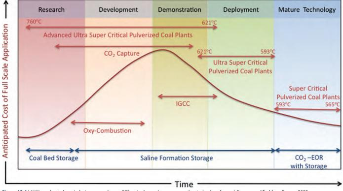
Figure 13.4 | Utility and petroleum industry perspective on CCS and advanced power generation technology for coal. Source: modified from Booras, 2009.
