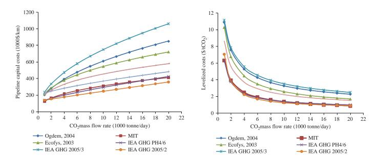
Figure 13.5 | Comparison of pipeline costs (a) and levelized costs (b) for a pipeline with a length of 100 km. Costs are reported in US<sub>2005</sub>\$. Source: McCollum and Ogden, 2006.
